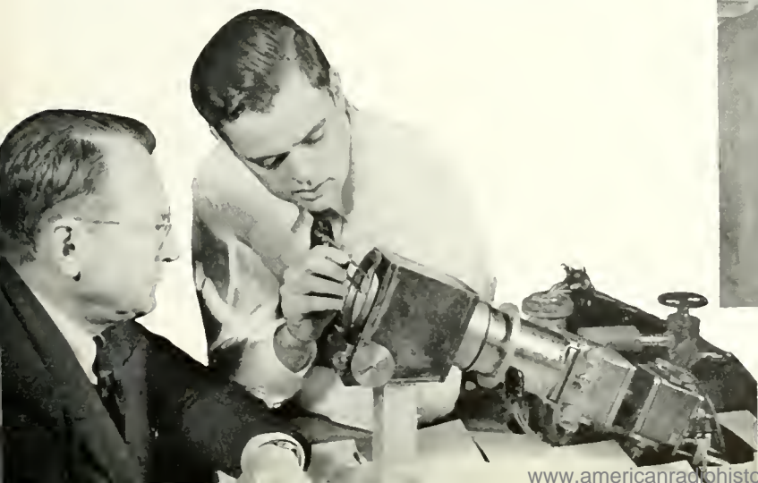
DR. V. K. ZWORYKIN (LEFT) AND DR. JAMES HILLIER AT WORK ON THE DESK-SIZE RCA ELECTRON MICROSCOPE, WHICH IS EXPECTED TO BE IN GENERAL USE SOON AFTER THE WAR.
