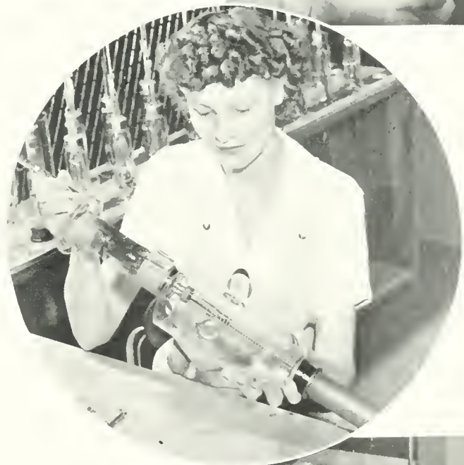
THIS GIRL OPERATOR INSERTS THE REBUILT MOUNT, OR INTERNAL STRUCTURE, INTO THE BULB-ANODE ASSEMBLY.
